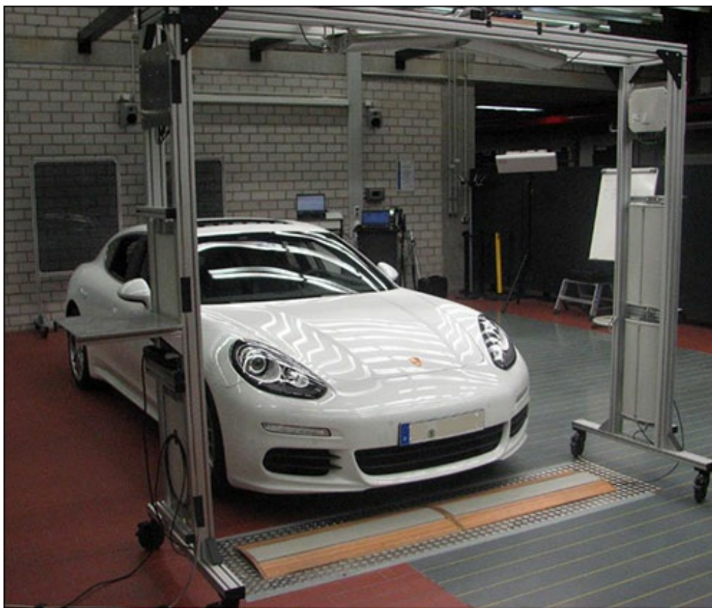
When testing is completed, a prototype vehicle is driven through a portal consisting of Kathrein RFID readers and antennas, to identify the vehicle's components by means of RFID tags.
