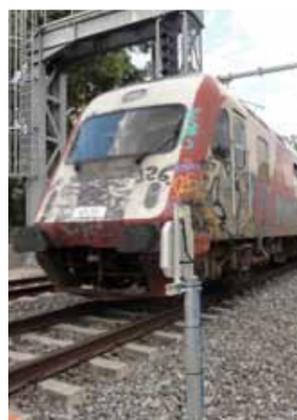
Kathrein RFID readers are installed along the railway line, which can identify trains at high speed
