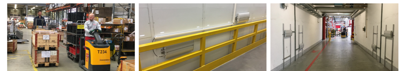
Figure: Supply with increased process quality. Empty RECA RFID KLT boxes are recognized as such and clearly read by the Kathrein RFID gates in only one direction of travel. They are thus automatically distinguished from the full boxes.
