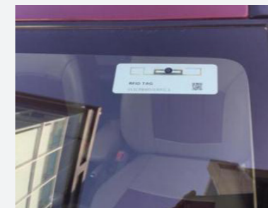
Illustration: Factory fitted RFID tags (given at co-driver side on front windshield)
