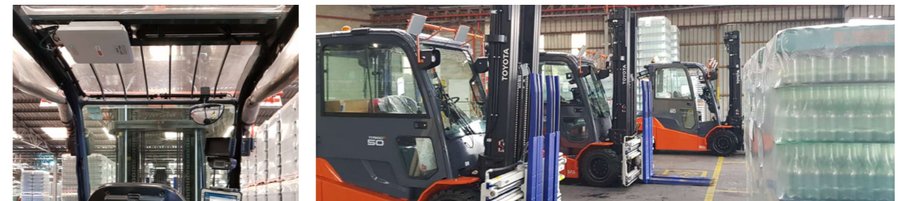
Figure: Integration of the reader in the driver’s cab of the forklift; forklift fleet with equipped RFID pallet detection system.
