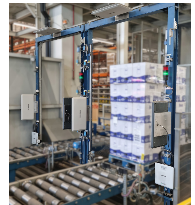
Figure: RFID gate/ RFID counting station, acquisition on two roller conveyors
