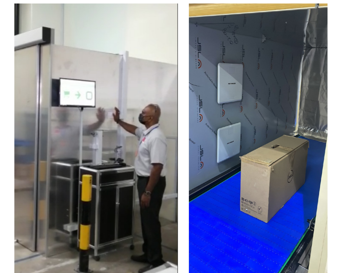
Illustrations: The materials are read and assigned in RFID chambers, among other things. The integrated software enables accurate monitoring of logistics processes.
