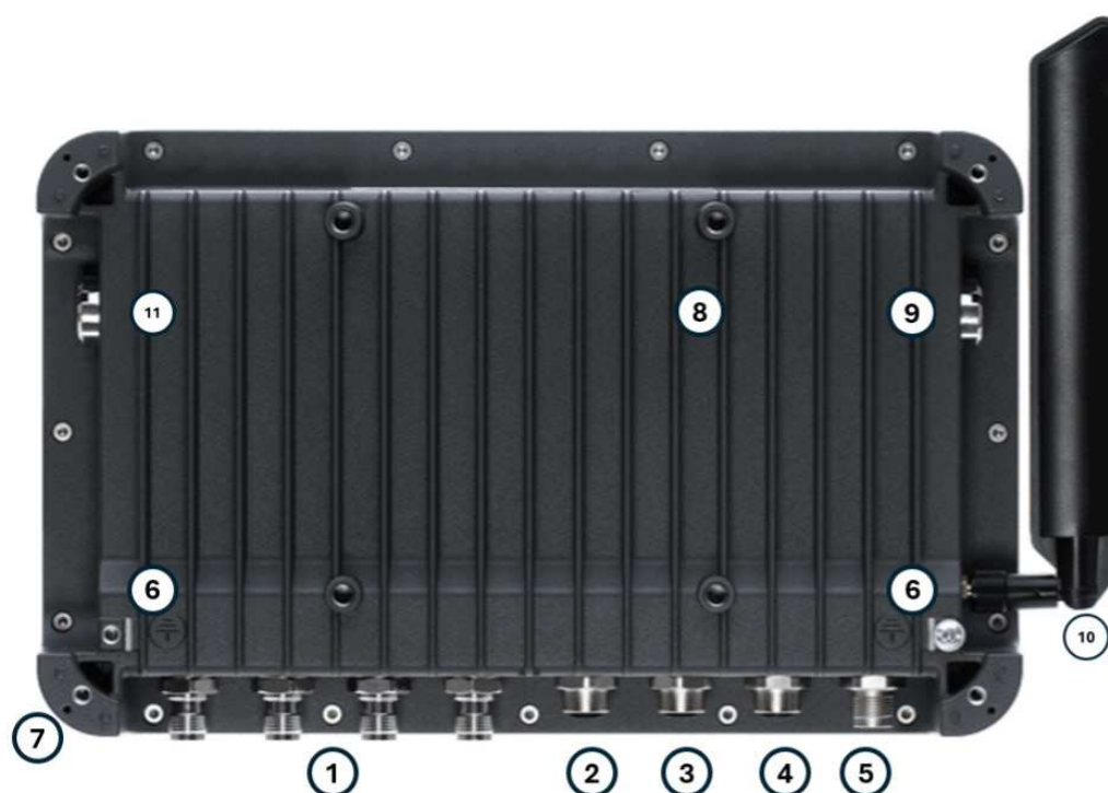
Fig. 11: RRU 4570 / ARU 3570 connections
